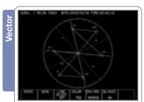
Vector display as 100/75% of multiformat color bars with I and Q axes displayed.
