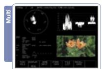
Multi Display of waveform, natural picture, status screen and vectorscope. Many other combinations are available.
