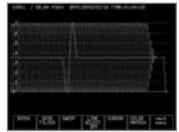
1080i/59.94 sweep of Y channel with horizontal x20 magnification applied.
